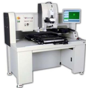
Extensive field experience and user feedback have resulted in the development of rework systems that exceed current and future industry requirements. Advanced rework software with intuitive 1-2-3 Go! operator interface and Auto Profile maximizes ease of use and throughput, while maintaining the inherent capability to rework today's most complex area-array components.
