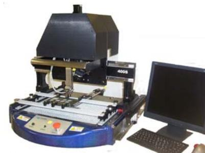
The VJ Electronix **400S** is a stand-alone, non-contact scavenging system for the automatic removal of residual solder from a rework site. With its automated X-Y motion, the 400S is pre-programmed to traverse the component site in the fastest and most efficient fashion, resulting in the optimum heat transfer to reflow the solder while minimizing thermal exposure. Dynamic Height Sensing (DHS) ensures optimum solderability for the replacement of a new component.
