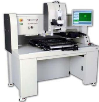
Also on display, the **Vertex Series A V130** X-ray system is production ready, offering superior uptime and unmatched value. Additionally, the system features a 130kv X-ray tube and total magnification of 1950X.
