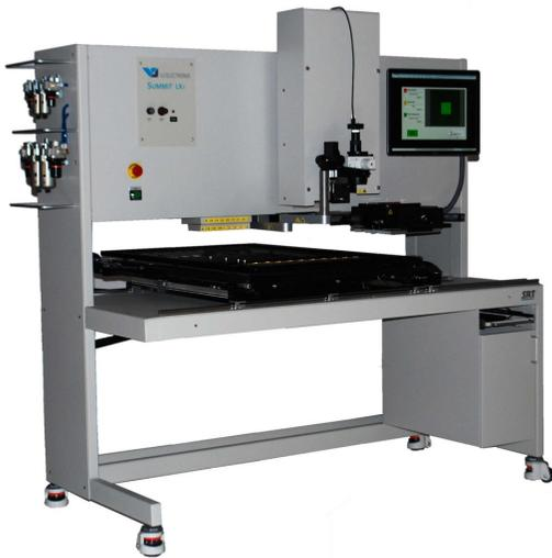
The Summit LX<sub>i</sub> carries forward the proven performance of the LX platform with a complete update to thermal process controls. Modeled after the SRT Micra and new Summit II, the LX<sub>i</sub>'s control system eliminates the affects of facility variations and supports more precise calibration, allowing process parameters to be readily shared between systems in multiple locations.
